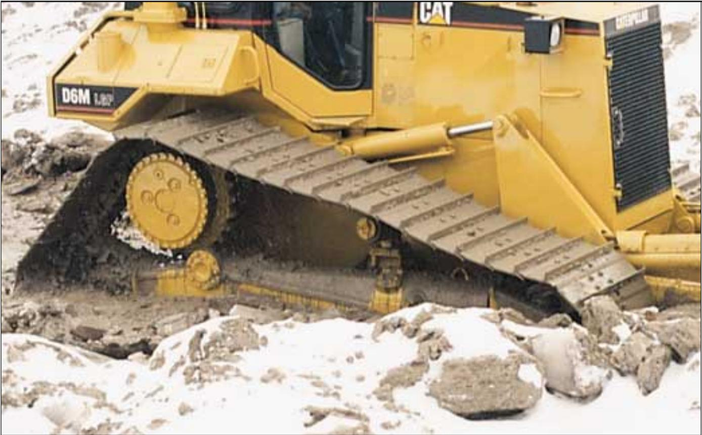
**Final drives and associated power train components** are raised above the work area, isolating them from ground-induced impact loads, as well as implement and roller frame alignment loads, extending power train component life.
