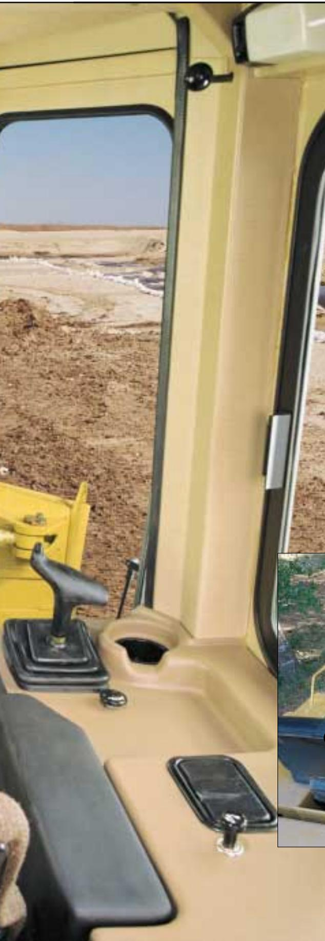
**1 Operator's station** provides excellent viewing area to blade and rear of machine. Optional isolation-mounted cab has reduced vibration and operator sound level below 79 dB(A) for comfortable operation. Standard cab is radio-ready with mounting brackets, AM/FM antenna and speakers.
